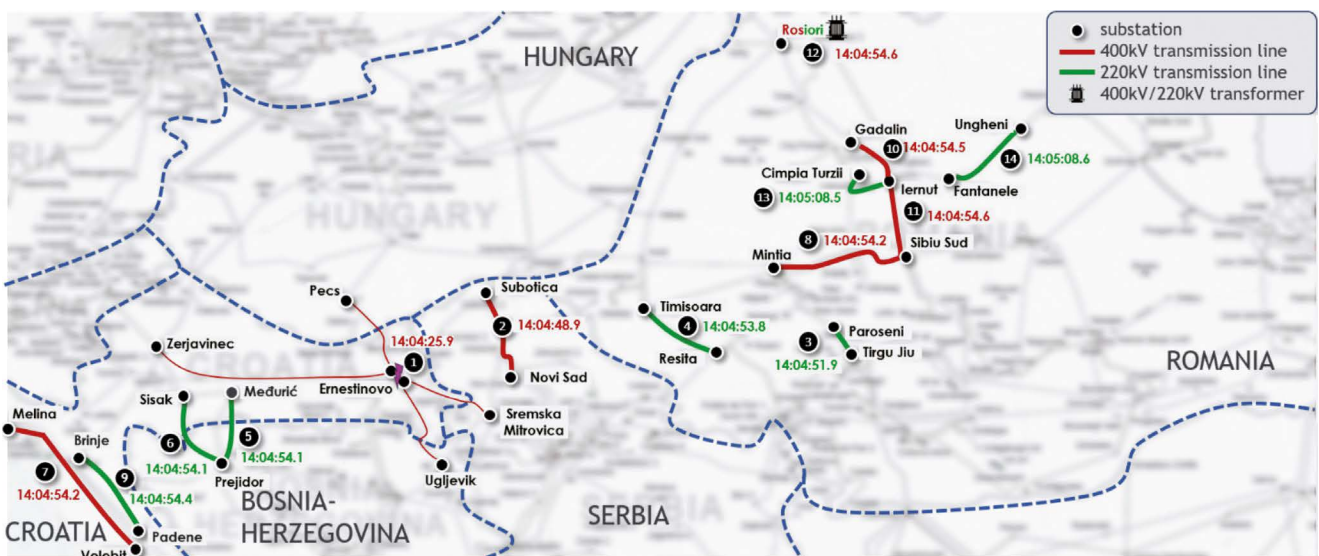
Figure 2.1: Geographical location of main tripped transmission system elements
